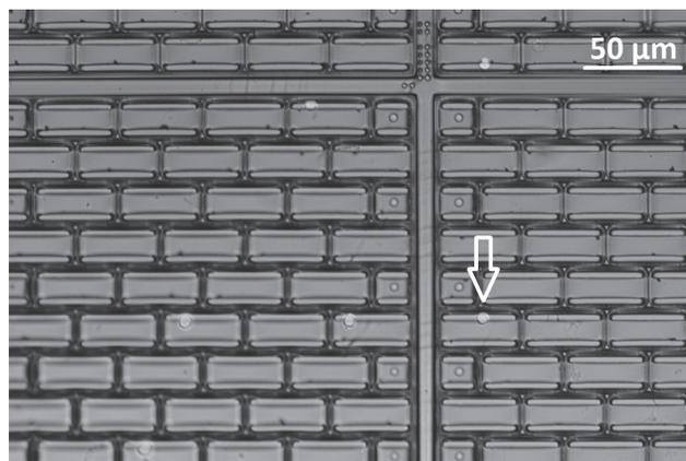
Figure 4: Device post-filtration (arrow points to a captured tumor cell).
