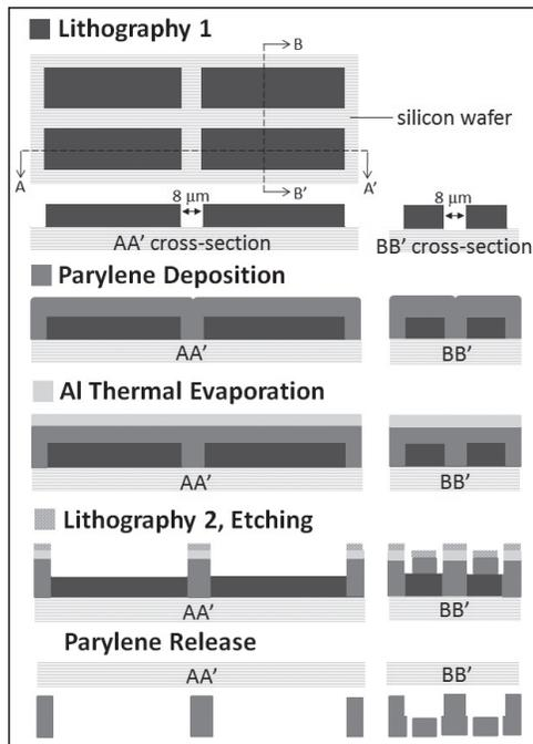
Figure 2: Micro-fabrication process flow.
