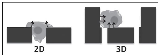
Figure 1: Forces on a trapped cell.
