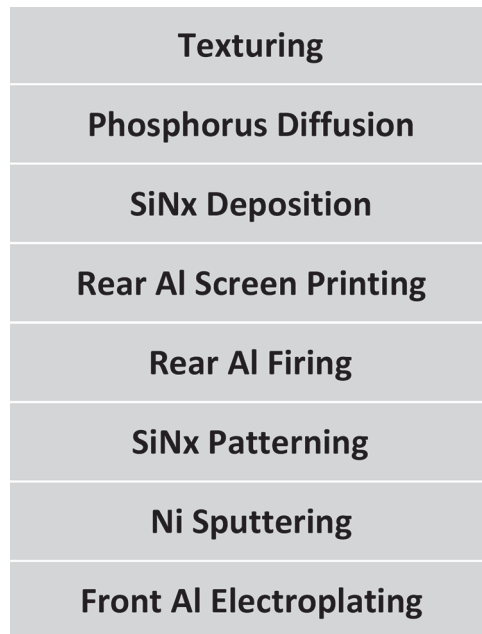
Figure 1: Process flow for the fabrication of this study's p-type solar cell. The silicon wafer was received with the first two steps already completed.
