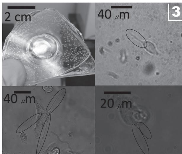
PDMS layer and cured at 100°C for two hours. After cooling, the sample was treated with an acetone mist via spray bottle and subsequently immersed in a methanol bath. Careful peeling of the support structure resulted in the production of a bounded membrane, which could be seen to oscillate in the methanol. The membrane was then carefully removed from the methanol bath [3].
