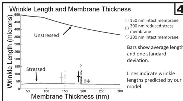
While we did find an upward trend in length and number of wrinkles as membrane thickness was reduced, our results indicated that our membrane was stressed as a side effect of our fabrication process. This residual stress substantially increased the minimum force required for cells to generate wrinkles, and likely reduces the device's power to differentiate between cells producing different ranges of force.
