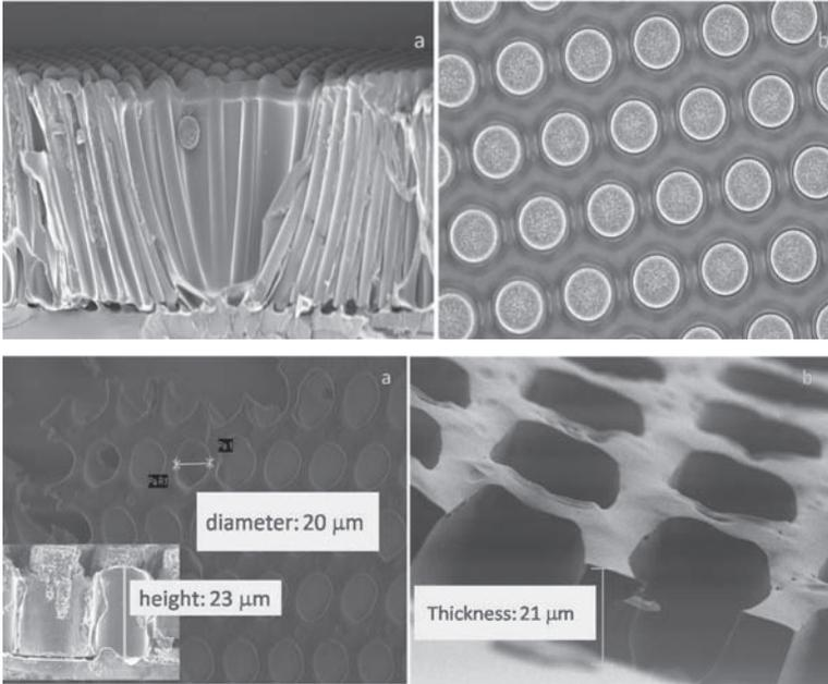
Figure 2, top: FE-SEM images of PI coated pillars (a) and RIE etched pillars (b). The pillar array of  $2.5\text{ mm} \times 2.5\text{ mm}$  that contained  $\sim 10^5$  pillars of  $20\text{ }\mu\text{m}$ -diameter,  $25\text{ }\mu\text{m}$ -high and a distance of  $5\text{ }\mu\text{m}$  between the pillars.
