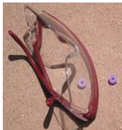
This pair of safety glasses blocks some UV light as seen with this simple set up.
