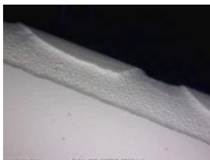
This picture shows the dot structures with the mask removed. The sidewalls are very sloped.
